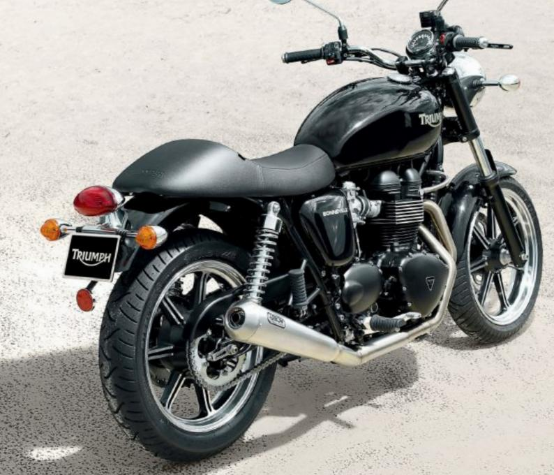
BONNEVILLE. REINVENTED. SO FIRE UP THE MODERN, FUEL-INJECTED, AIR-COOLED 865CC PARALLEL TWIN. LISTEN TO THE RICH SOUND FROM THE UPSWEPT MEGAPHONE EXHAUST. THAT'LL PUT A SMILE ON YOUR FACE. A LOWER, NARROWER SEAT FOR A MORE SECURE FOOTING AND BALANCE AT A STOP, AND A MORE APPEALING, RELAXED RIDE. 310MM FRONT DISC. 255MM REAR DISC. A CLASSIC. REBORN.
